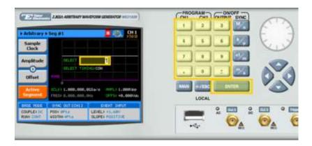
3. When selecting a numeric attribute for modification, modify the displayed value using the dial or the cursor keys, or by entering the value using the numeric keypad. Press ENTER to save the modified parameter value.
